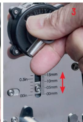
**3** - Rolling thickness is given in mm and inches below the thumbwheel. Each thumbwheel notch number gives a lamination thickness for precise adjustment. See page 6-7 for correspondence between notches and thickness in mm.
