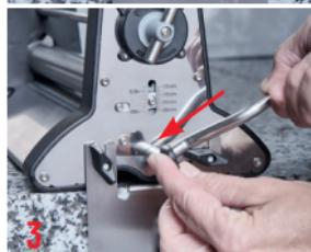
**3** - Unscrew the crank fixing screw, insert the crank into the hole provided on the rod and retighten the screw firmly.
